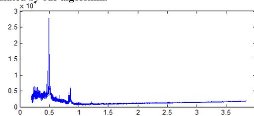
Figure 2. Example of MALDI MS mass spectrum after baseline correction using the baseline correction routine in the Data Explorer software. The overall intensity has decreased in low mass to charge ranges, but the spectrum seems to rise in the high mass to charge ranges.
