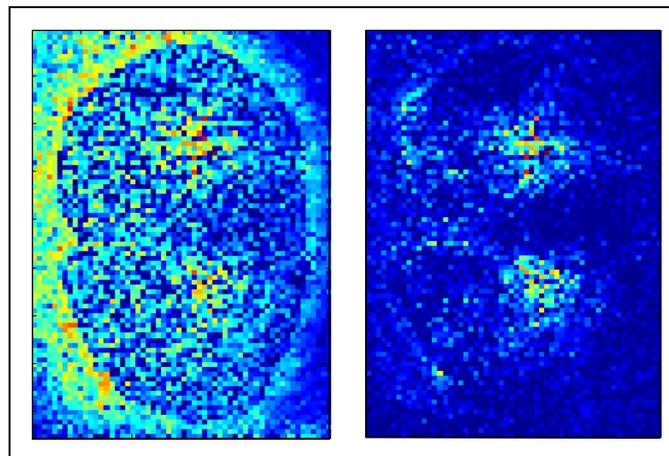
**Figure 3.** MALDI MS image of a male mouse brain created by averaging over a mass to charge range in each of the spectra in the dataset. The pixel colors are assigned linearly based upon ion count, using a blue-cyan-yellow-red color scale. Dark blue represents the lowest intensity and red represents highest. The image on the left is computed using MALDI data that has not been baseline corrected, and the image on the right was constructed after baseline correction
