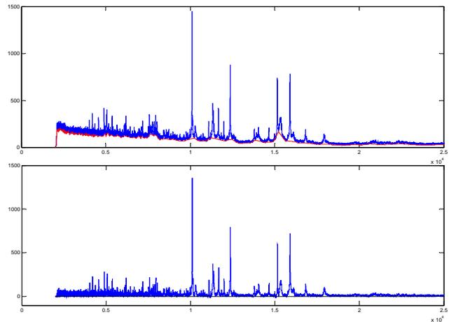
**Figure 11.** The top spectrum shows mass spectrum with the baseline calculated by linear interpolation seen in red. We see at the mass to charge value of around 15,000, the baseline rises up into the peak. By having a baseline at this point, important peak information is lost after baseline subtraction as seen in the second spectrum.
