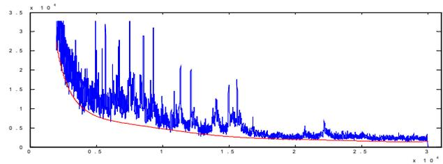
**Figure 12.** Example of spectrum shown in blue and the resulting baseline shown in red found by fitting polynomial through the minimum of a window.
