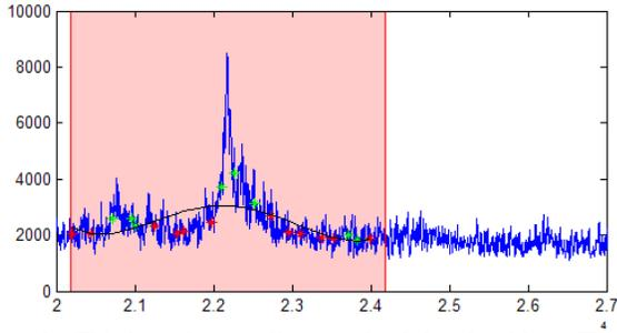
**Figure 9.** This is an intermediate result of the algorithm. The local area has expanded, but there are still too many median points more than epsilon above the polynomial. Median points epsilon above the polynomial are shown in green, the rest are shown in red.
