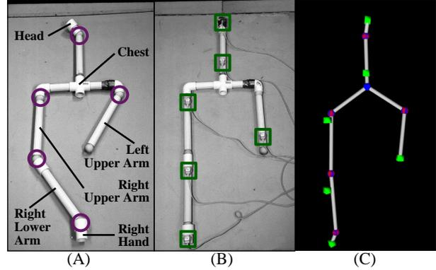
Figure 5: Wooden mechanical linkage. (A) Labels indicate the terms that we used to refer to the body parts; circles highlight the joint locations. (B) The motion capture sensors (highlighted squares) have been attached to the linkage. (C) The model computed automatically from the motion data using our algorithm. The joints are shown with spheres, and the sensors with cubes. Links between joints are indicated with cylinders.
