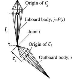
Figure 3: Joint diagram showing the location of the rotary joint between bodies  $i$  and  $j = P(i)$ . The location of the joint is defined by a vector displacement,  $\mathbf{c}_i$ , relative to the coordinate system of body  $i$ , and a second vector displacement,  $\mathbf{l}_i$ , in the coordinate system of body  $j$ .
