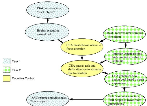
Fig. 6. Process flow of the cognitive control experiment
